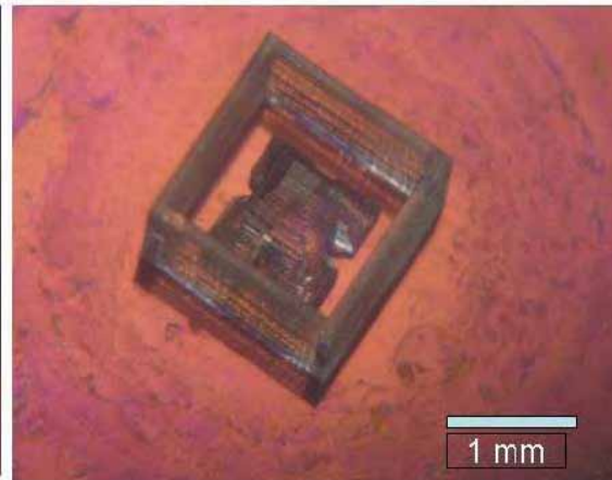
Pyramid with 1mm size fabricated inside a tank of size 1.6mm Height of the structure is 750 \mu\text{m} 15 layers
