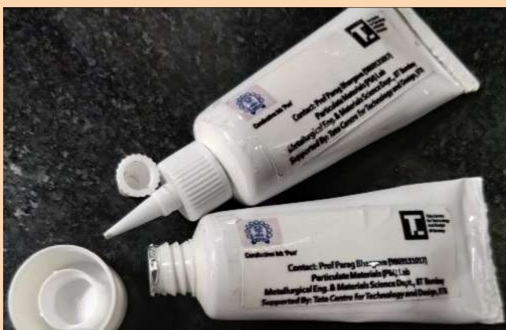
Pictures of tube filled with silver paste for making circuits on paper for educational purposes
